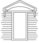
Inappropriate entrance alteration: paneled door to flush door; closure of sidelights
