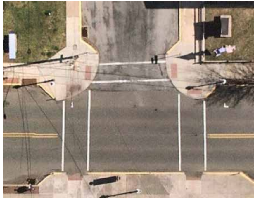
Below: Aerial image of the curb bumpouts at Main & Bank Street
